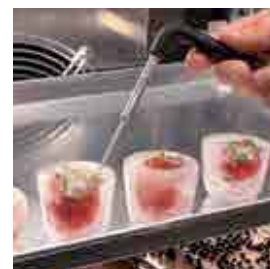
Sonda rilevamento temperatura Probe to survey the core temperature of the product
